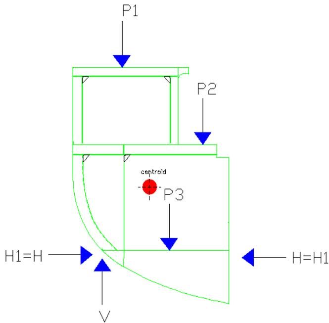
**Line of action of force & shear center should coincide**
